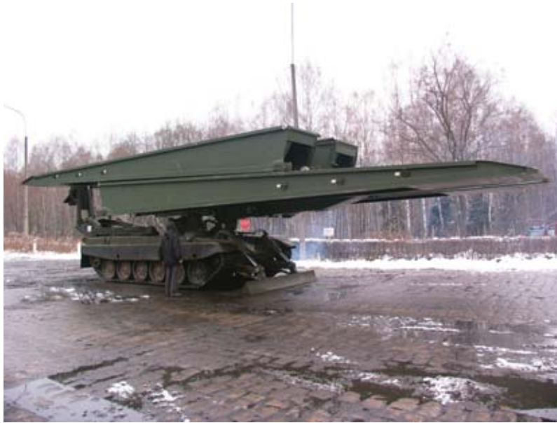
Fig. 5. PMC-LEGUAN bridge during factory tests
