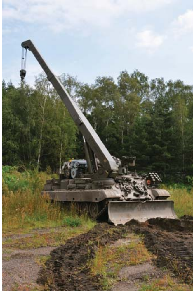
Fig. 3. WZT-4 during terrain tests (interchangeable power pack is visible on the loading box)
